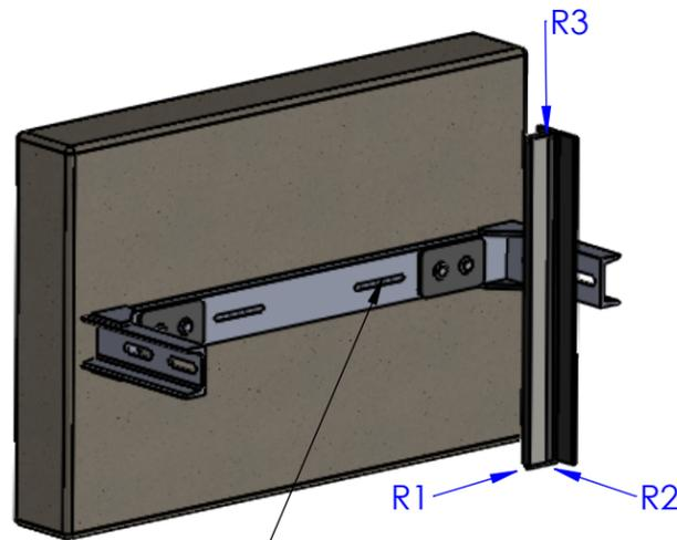
ATTACH VIA 3/8 X 4" LAG BOLTS FOR WOOD OR 3/8 x 5" WEDGE ANCHOR FOR CONCRETE
