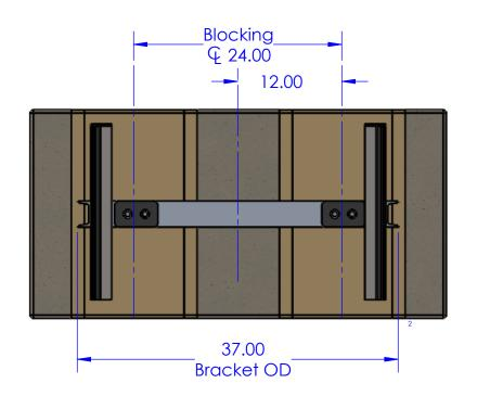
Double stacked 2x12 with 2x4 end caps running the full vertical length of the rail support wall.
