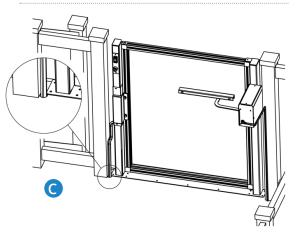
**TIP:** You can install the upper gate later during the install process because you have to make sure it is aligned with the platform side walls.
