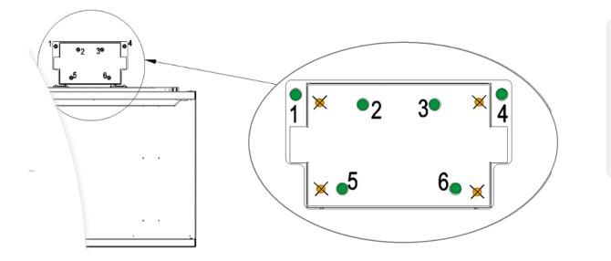
**TIP:** Hide the acme screw bearing when drilling holes and clean dust after the drilling to avoid having dust inside the bearing which could cause noise when using the platform.
