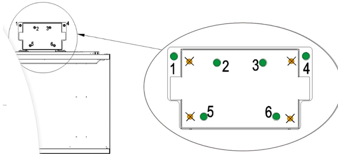
**TIP:** Hide the acme screw bearing when drilling holes and clean dust after the drilling to avoid having dust inside the bearing which could cause noise when using the platform.
