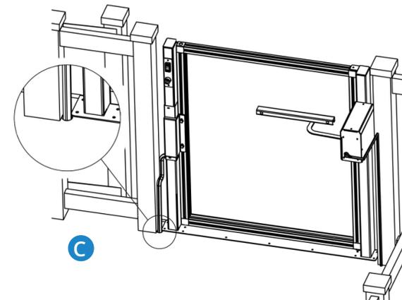
**TIP:** You can install the upper gate later during the install process because you have to make sure it is aligned with the platform side walls.
