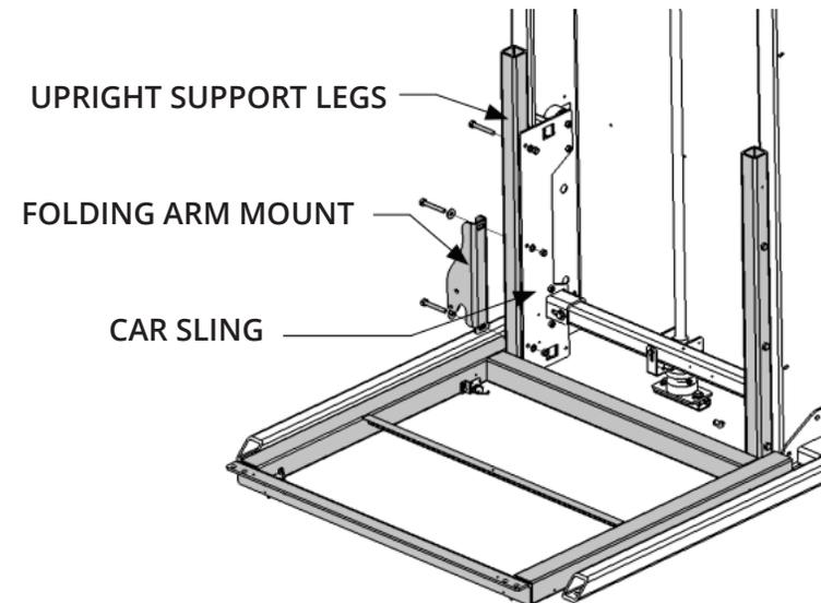
**TIP:** Secure traveling cable on the side of the car sling.
