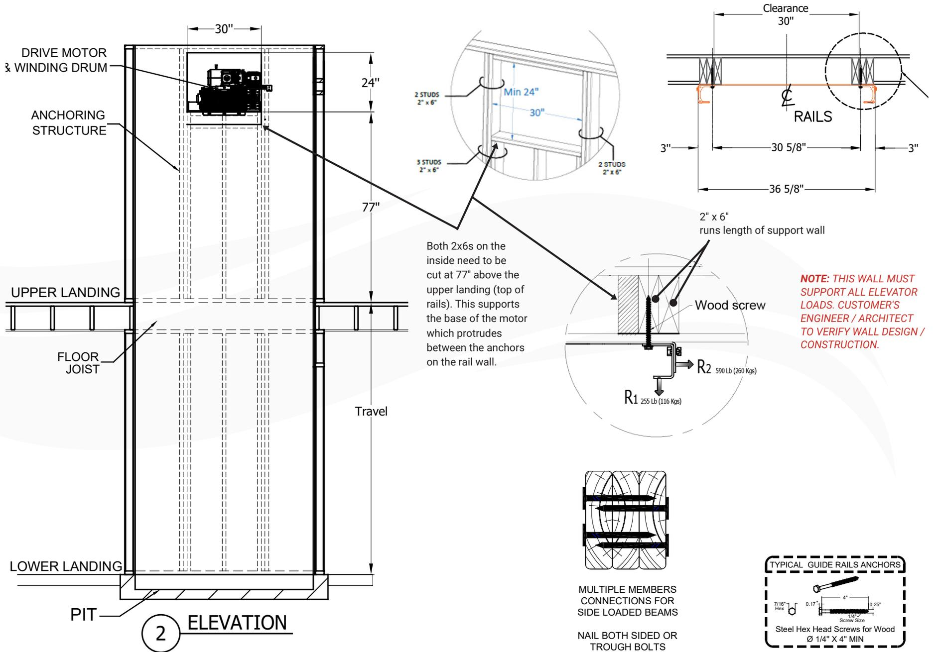
Both 2x6s on the inside need to be cut at 77" above the upper landing (top of rails). This supports the base of the motor which protrudes between the anchors on the rail wall.
