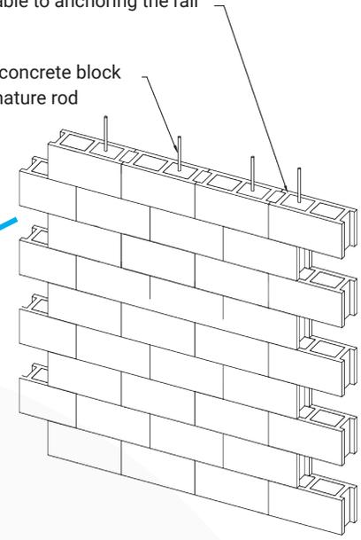
Each block cell of the supporting wall must be poured with concrete, for to be able to anchoring the rail
