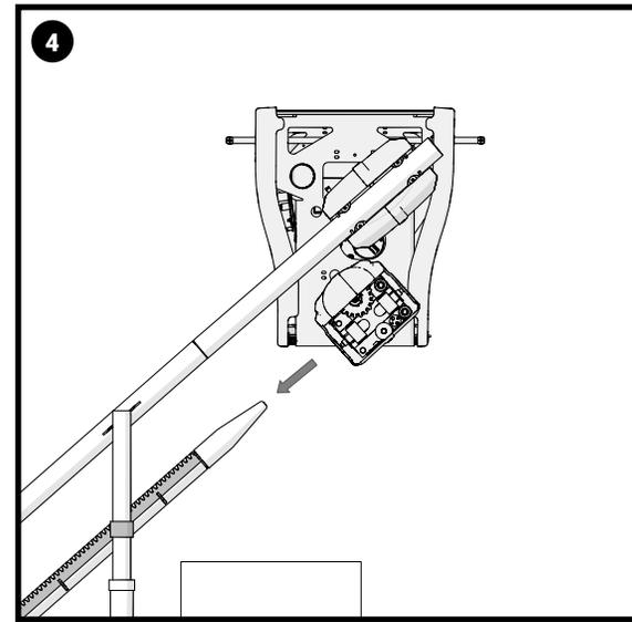
With the loading bar inserted, gently guide the carriage and bottom skate onto the loading cone, ensuring correct alignment to avoid damage to the bottom skate.
