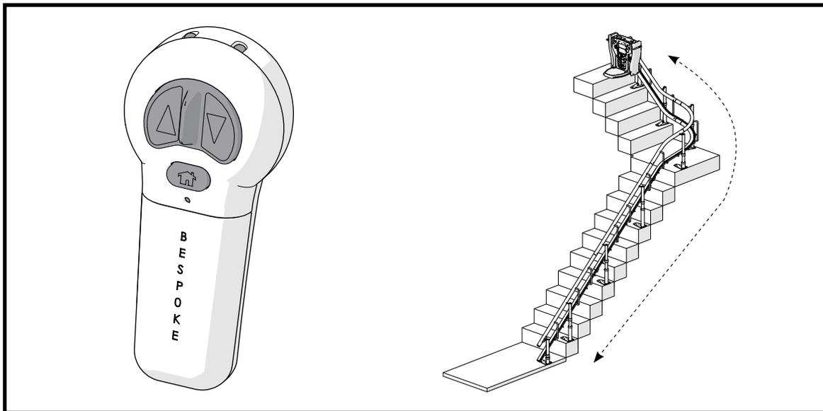
The carriage can now be moved using the remote controls.
