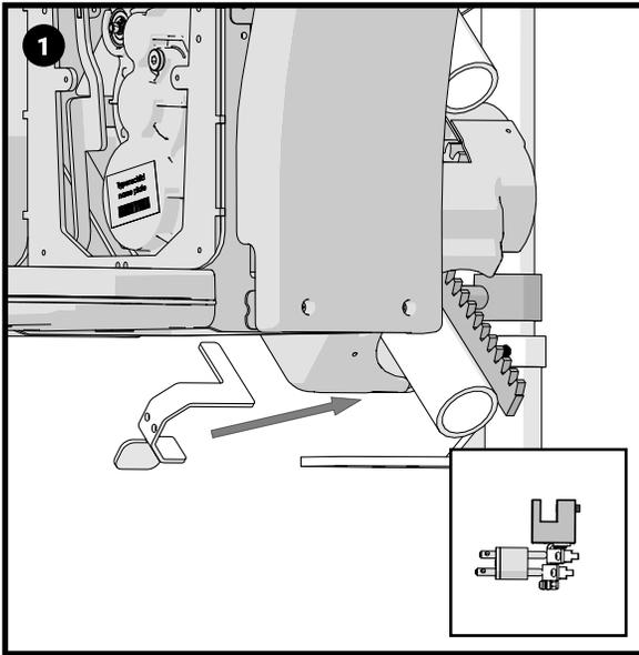
To mark the position of the end stops, run the carriage down so that the charge pins are engaged with the charge point at the bottom of the rail.
