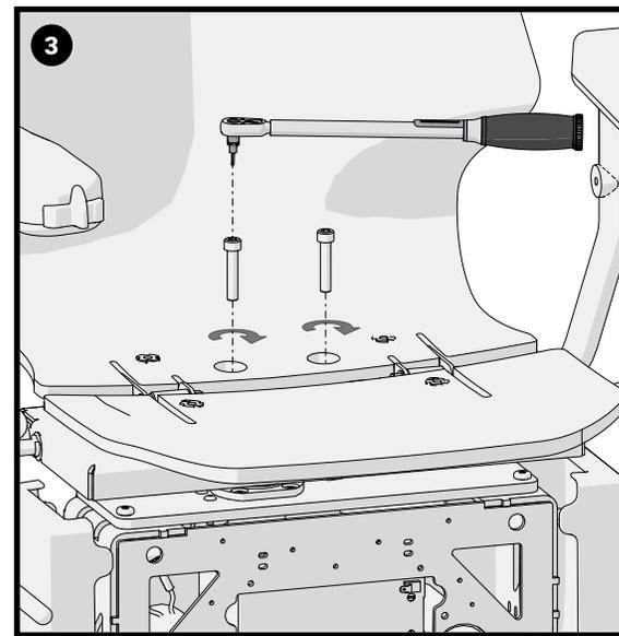
Attach the seat by using the M8 x 40mm bolts through the rear section of the seat into the seat swivel boss. Tighten to 22Nm.
