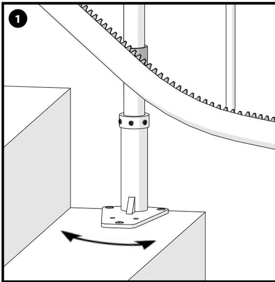
Once the final rail position checks are complete the rail can now be fixed in position. Straighten up the footplates on the step ready for fixing.
