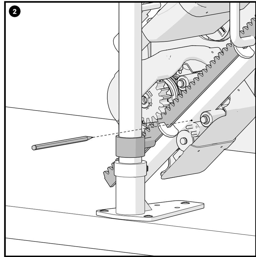
With the carriage in the desired position, stop the carriage and mark the position of the of the charge pins on the bottom skate.
