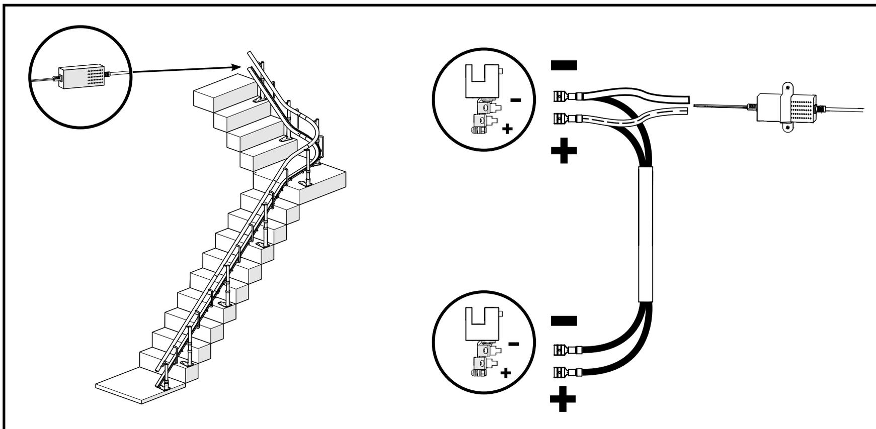
If the charger is connected to a power supply on the upper level of the stair lift use the diagram to correctly connect the power charger to the charge points.
