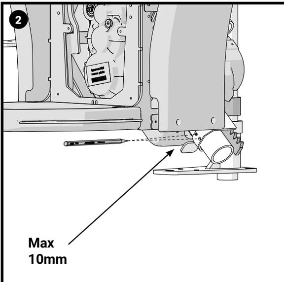
To ensure the carriage still charges should the end stop engage the safety edge, the maximum distance from the end stop to the bottom skate cover is 10mm.
