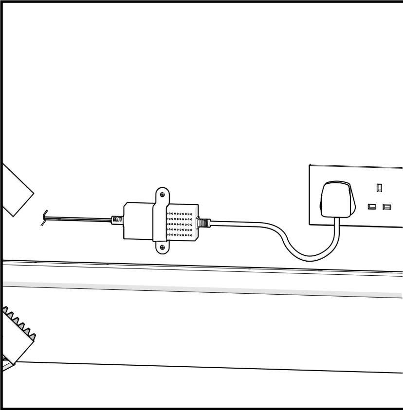
Turn 'ON' the charger at the mains. (If an intermediate charge point has been installed, move the carriage down the rail until it is past this point prior to turning on the charger).
