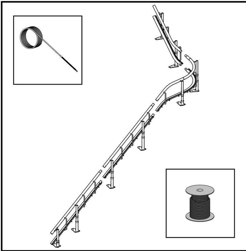
Start with positioning the cable supplied with your curved stair lift near the bottom rail section of the stair lift.
