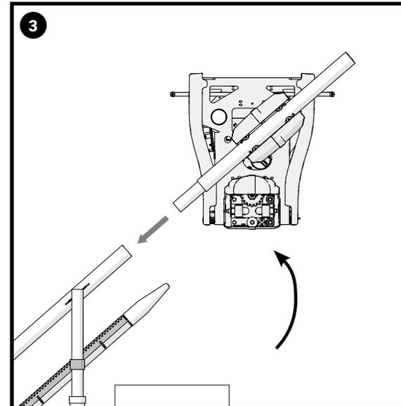
Support the carriage by the loading bar and insert the smaller end into the top tube of the rail. Be careful to avoid the carriage slipping down the loading bar.
