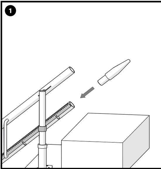
To begin loading, take the carriage to the top of the stairlift along with the loading cone and loading bar.
