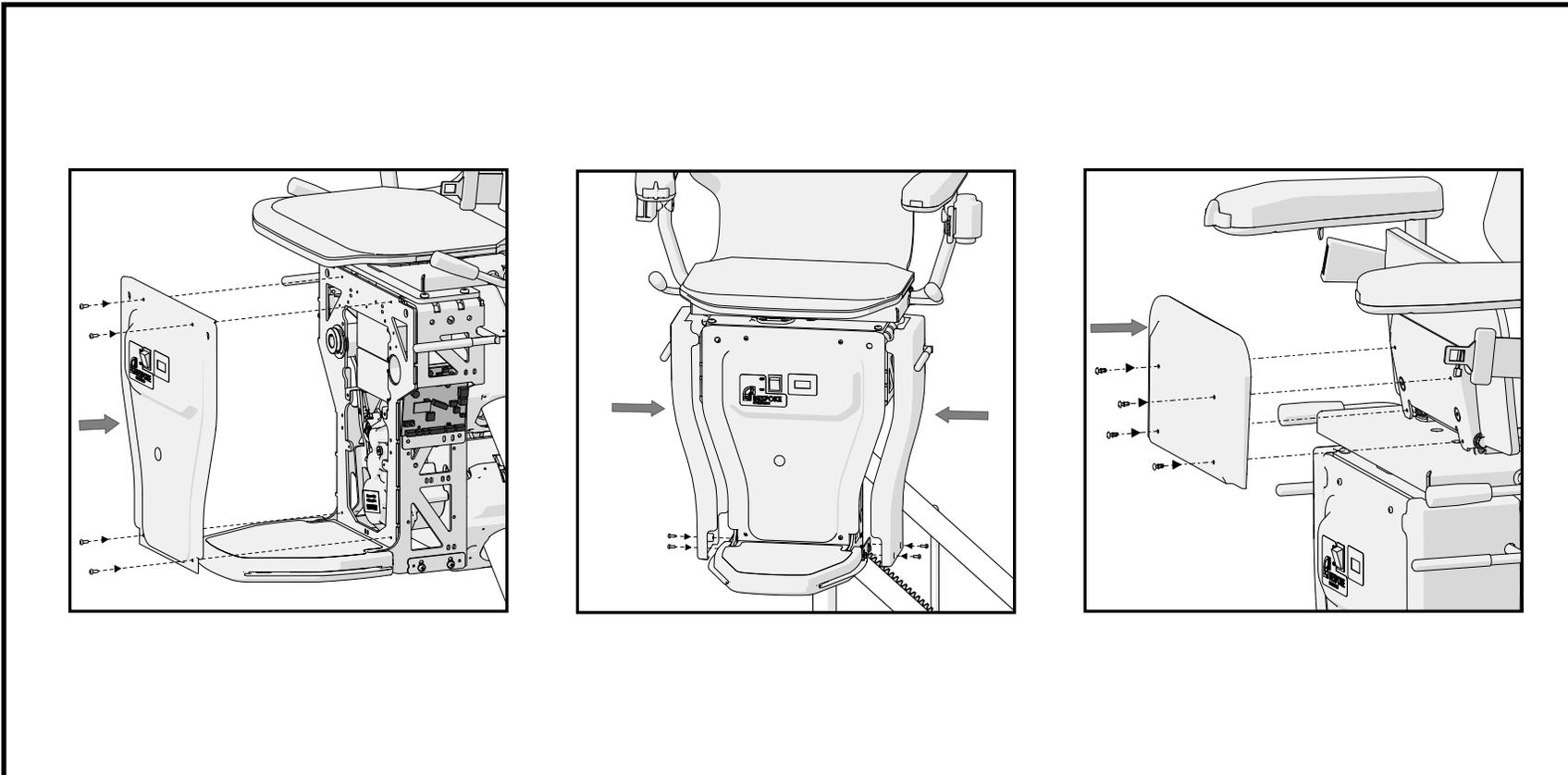
Replace the front and side panels using the screws removed earlier.
