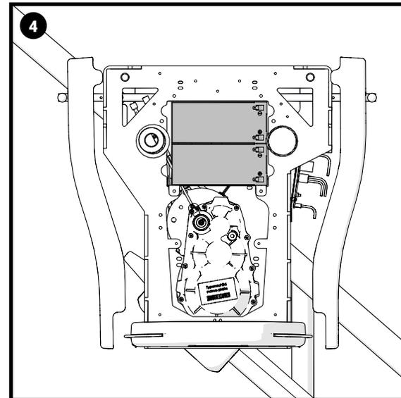
Once the batteries are in the correct position, they can now be connected to the carriage.
