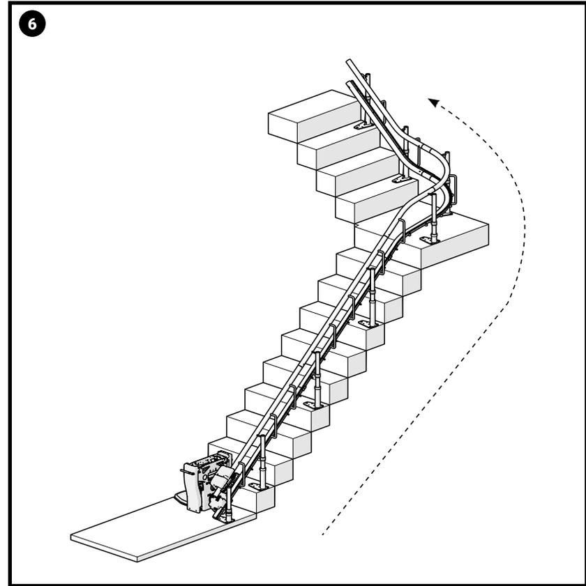
Now run the carriage to the top section of the rail, ready for installing the top end stop.
