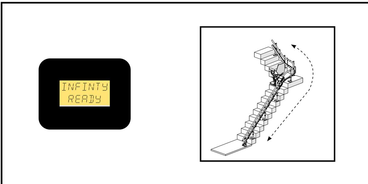
The programming is now complete and the display will read **'INFINTY READY'**. Test the rail by running the stair lift back down to the bottom charge point and then the top. The lift is now programmed.
