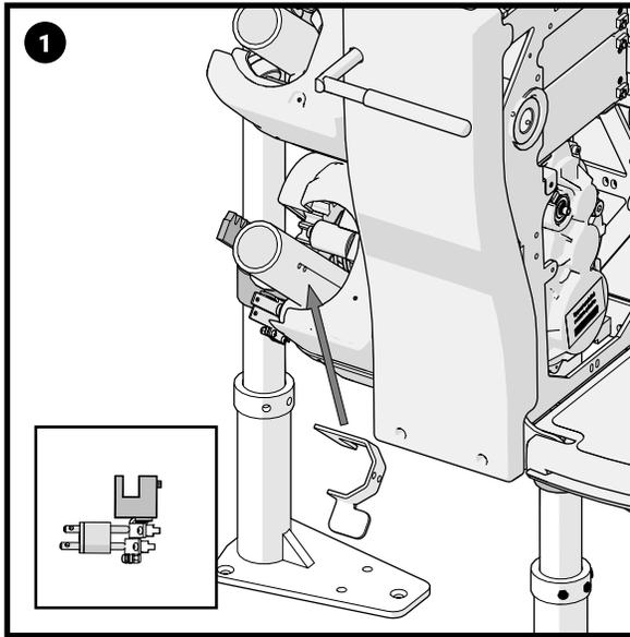
Run the carriage upward, so that the charge pins are engaged with the charge point at the top of the rail.
