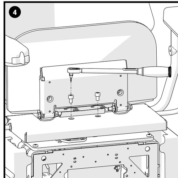
Lift the flip section of the seat to enable insertion of the M8x12 screws in the front section. Tighten to 22Nm.
