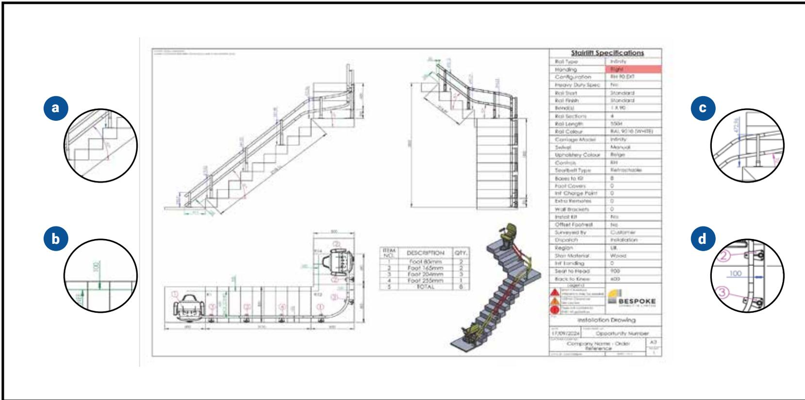
1 - 3 Staircase elevations, staircase dimensions, leg heights and positions
