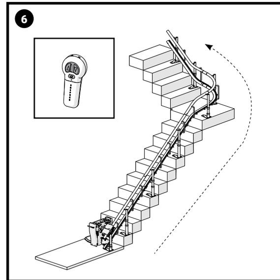
Move the carriage to the top of the rail to the desired terminal location.
