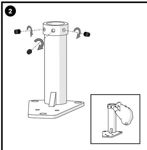
Before placing on the stairs, insert 3x M6 grub screws into each base.
