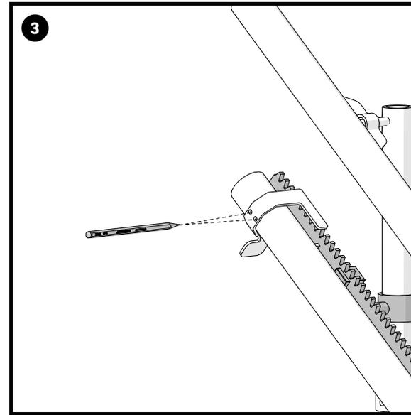
Mark the position of the upper end stop in the correct location.
