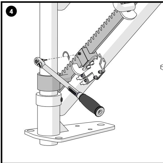
Tighten the charge point securely at the bottom of the rail to 10Nm.
