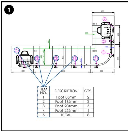
The number on the plan view of the installation drawing relates to the item number on the leg table. Item numbers are different sized bases.
