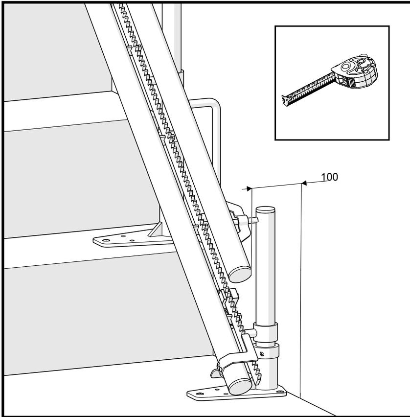
Check the clearance measurement of the rail at the bottom against the wall or closest obstruction. This should be no less than 100mm.
