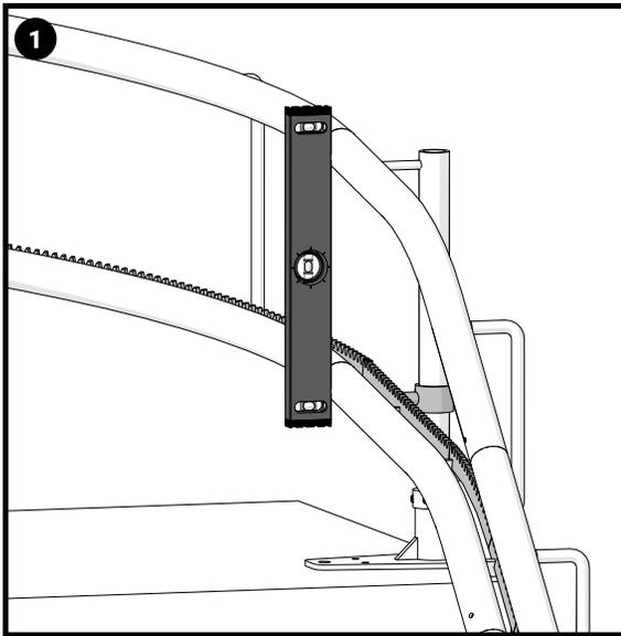
If the rail is out of level it can be adjusted by raising or lowering the base opposite to correct.
