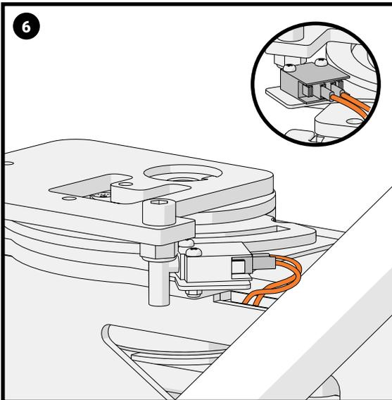
Now connect the orange cables to the powered swivel unit.
