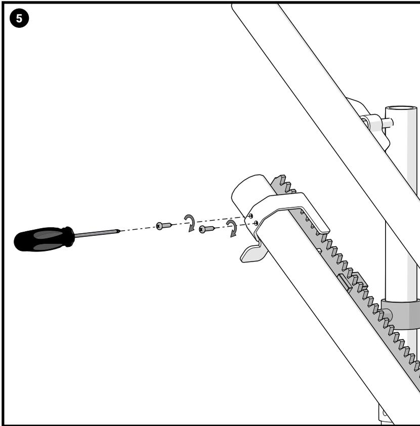
Attach the end stop using the self tapping screws provided.
