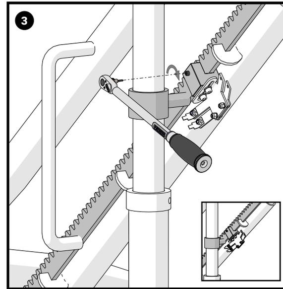
Tighten the charge point securely to the bottom rail, to 10Nm.
