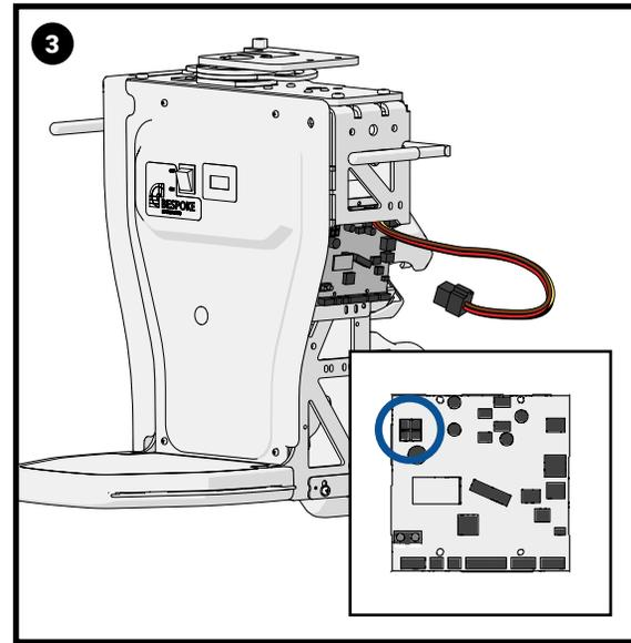
Connect the other end of the auxiliary cable to the main PCB AUX connection.
