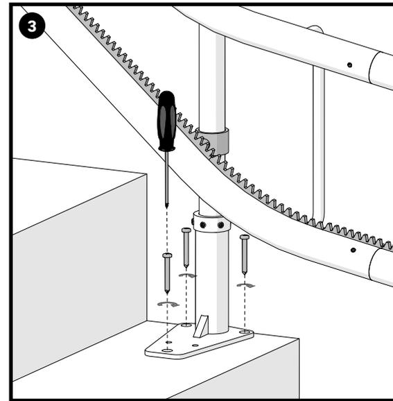
Fix the base to the stair tread using (3x) M10x50mm screws, ensuring they are fixed neatly.
