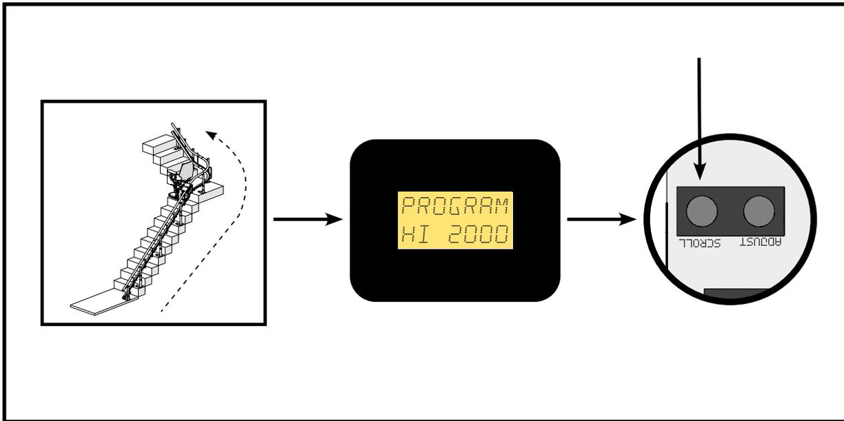
Once the bend(s) speed is programmed, using the remote control, move the stair lift up the rail until it reaches the top charge point. The display will read a higher number as the stair lift travels. Press and hold the **'SCROLL'** button.
