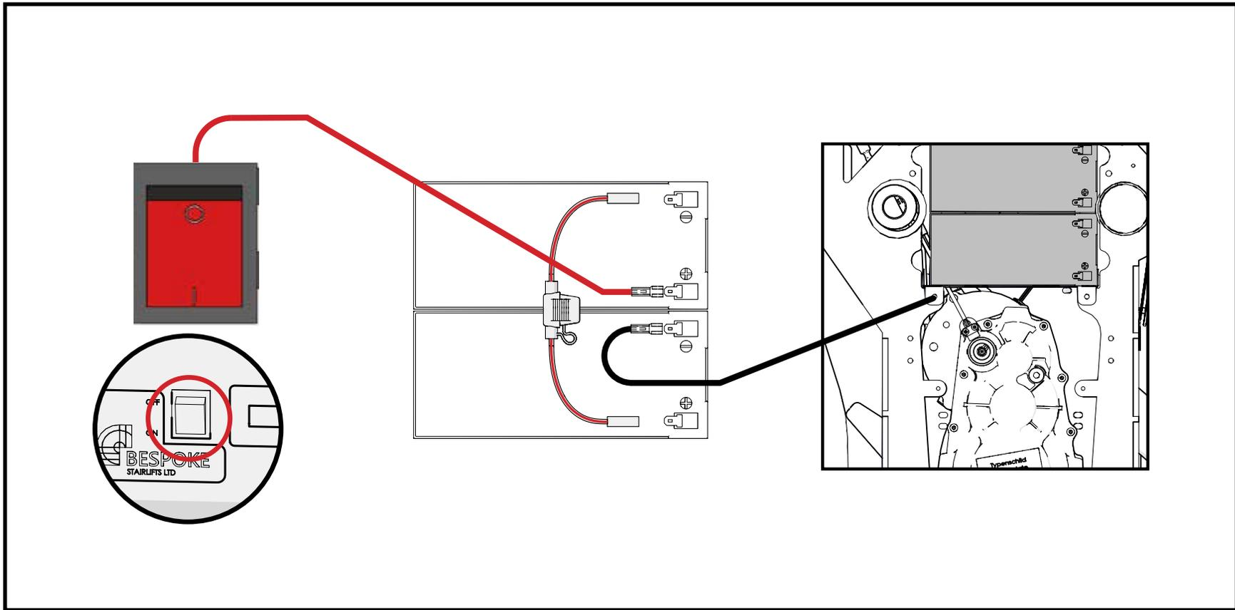
Connect the red cable from the main power switch to the '+' terminal on the top battery.
