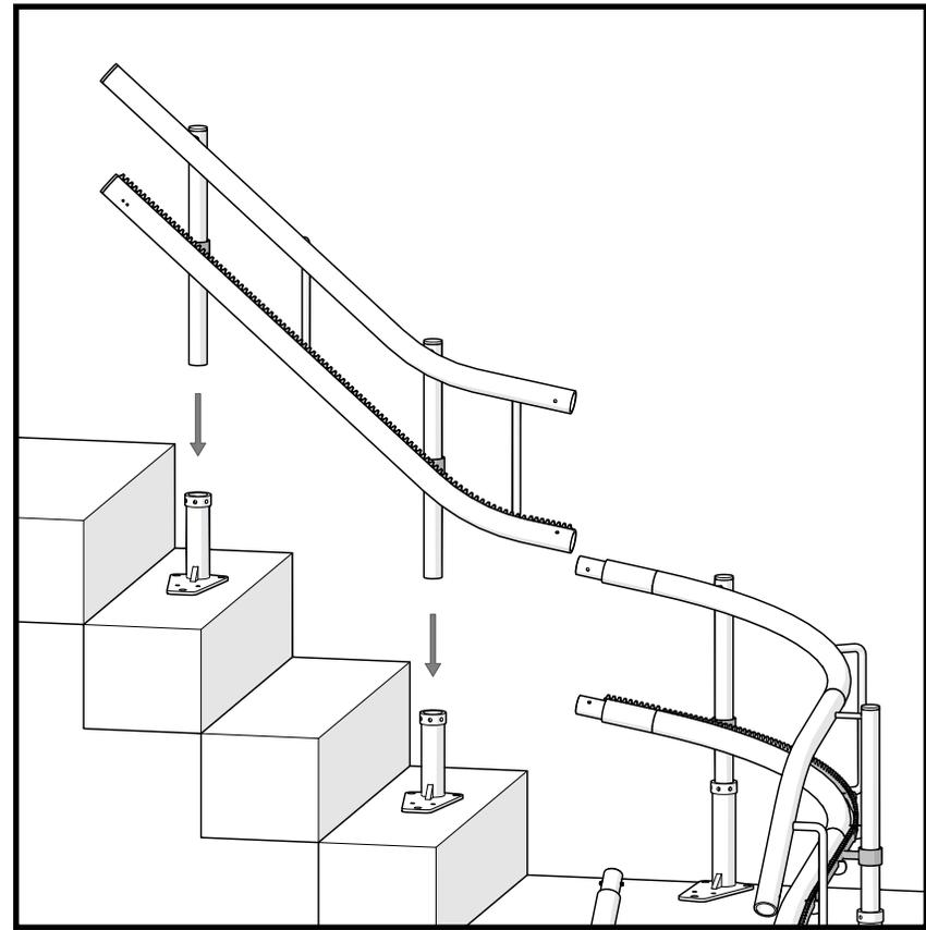
Continue to do the same for the remaining sections until all the sections are in the correct bases and in their correct position on the stairs.
