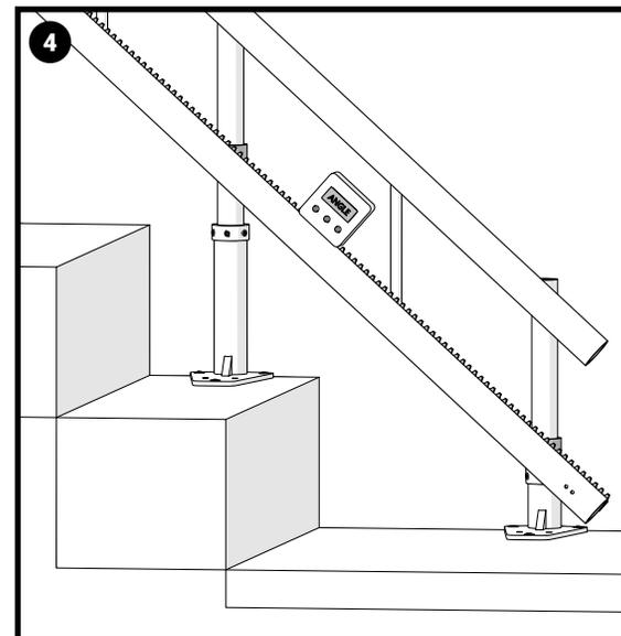
Check the angle corresponds closely with the install drawing, once complete we can fix the rail to the stairs.
