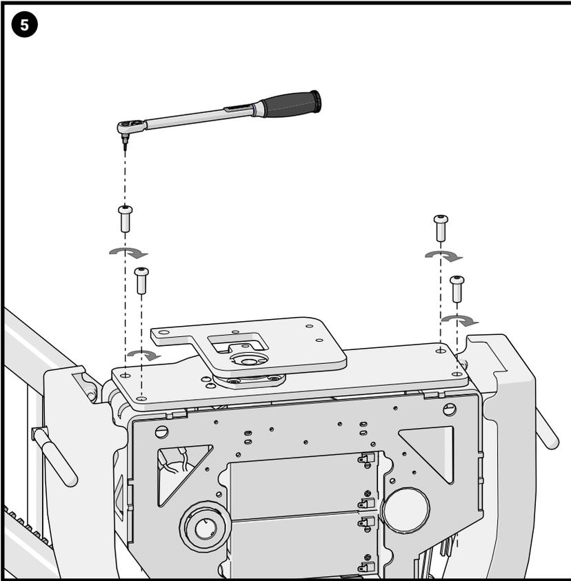
Secure the Swivel Assembly to the Carriage with the 4xM8 screws and tighten to 30Nm.
