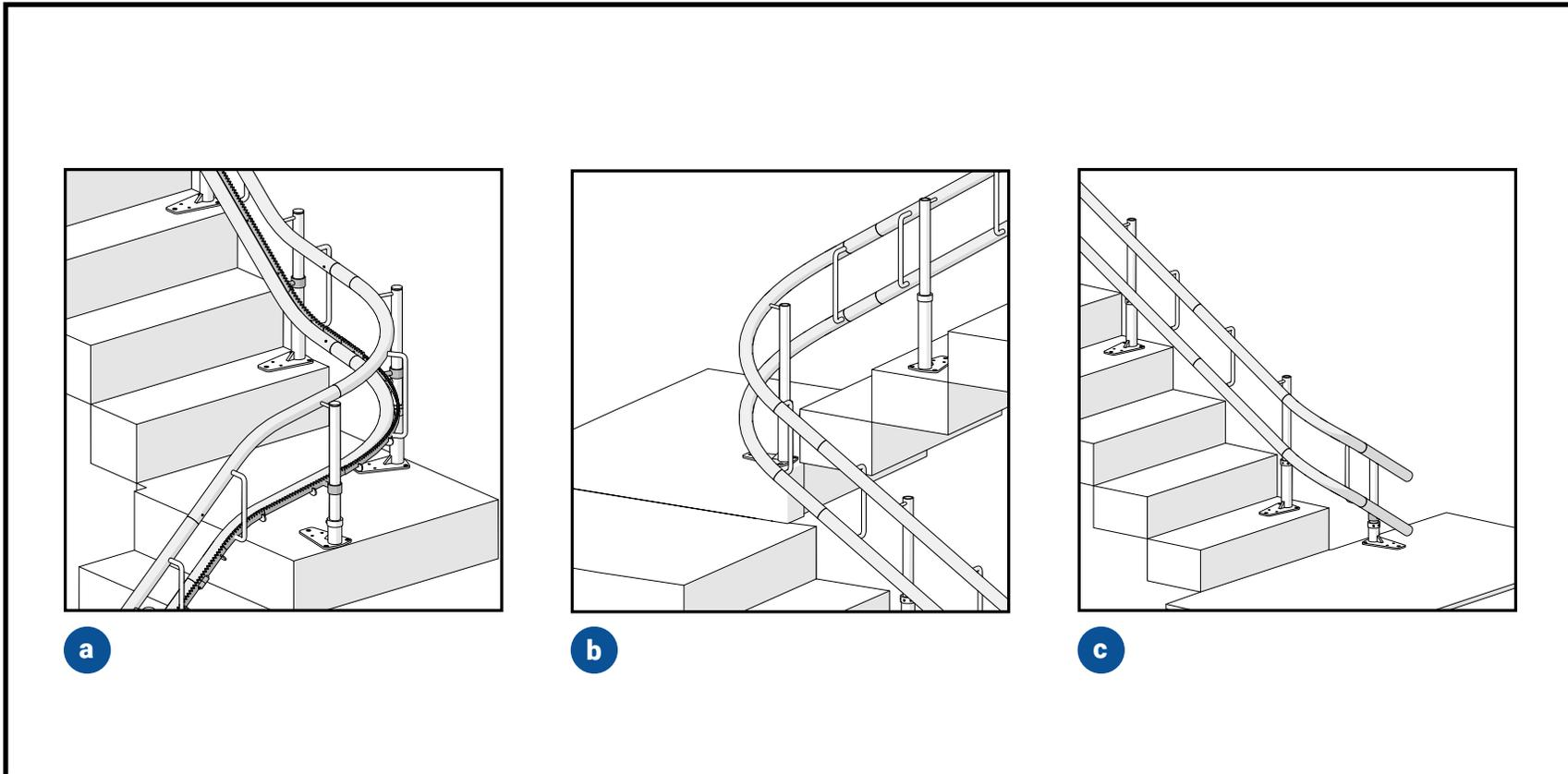
Certain types of rail require the speed of the stairlift to slow down to ensure safe travel. Internal bends require this whereas external travel bends do not.
