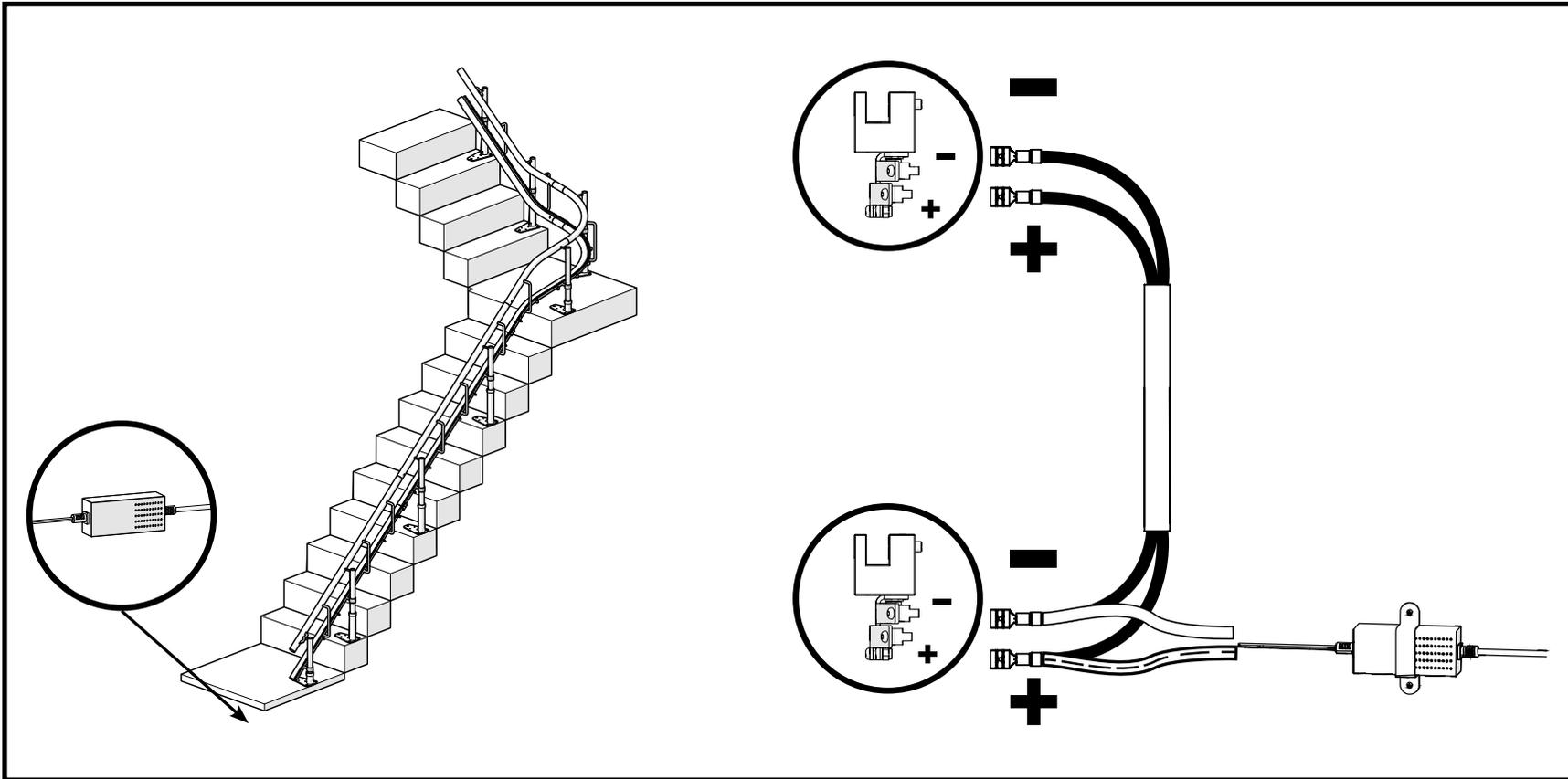
If the charger is connected to a power supply on the lower level of the stair lift use the diagram to correctly connect the power charger to the charge points.
