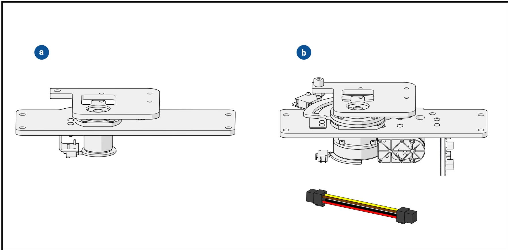
The next step is to mount the swivel. Select which swivel type and move onto the correct section for installation details.
