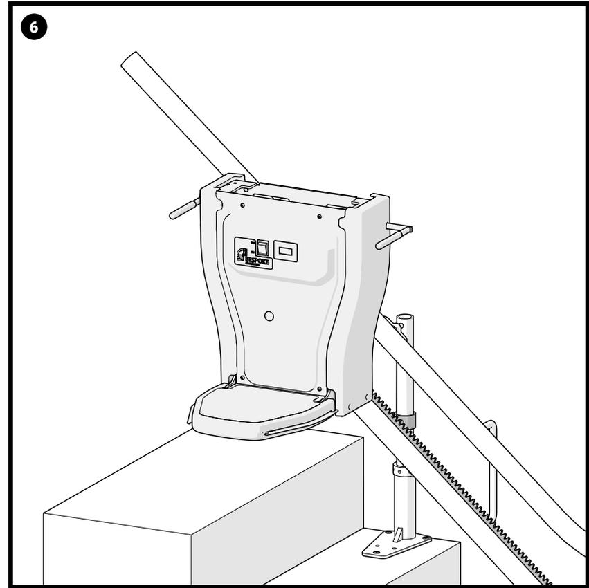
The carriage is now loaded onto the rail.
