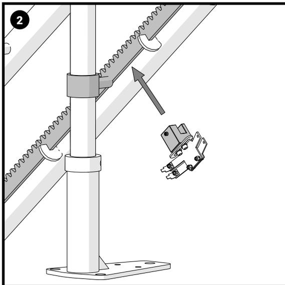
Switch the carriage on and move the carriage down, away from the charge point location. Attach to the racking using the grub screw.
