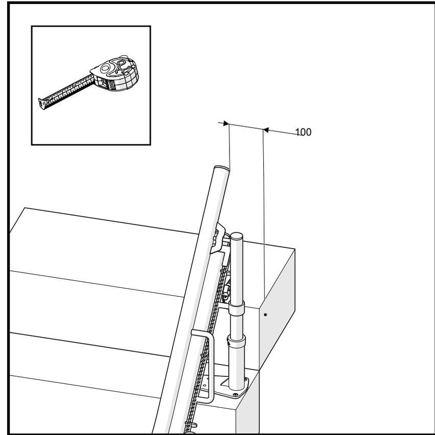
Work your way up the rail and position the straight sections the same 100mm from any wall or obstruction.
