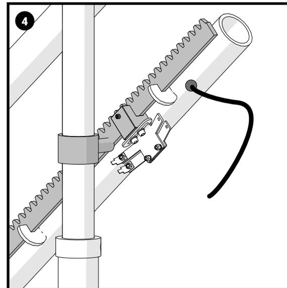
The top charge point is now secure. Now feed the cable through the hole in located near the top of the rail in preparation for connection.
