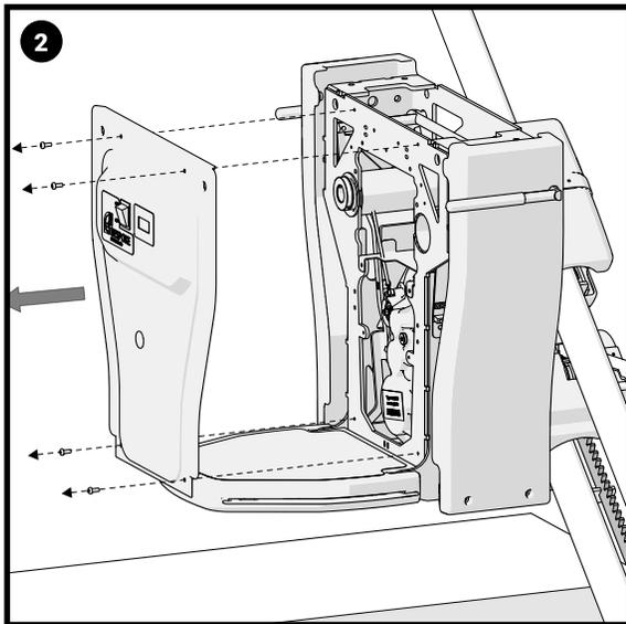
Carefully remove the screws from the front panel to enable the installation of the batteries.
