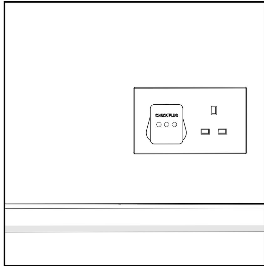
Using a mains socket tester to ensure the site wiring is safe and free from faults.
