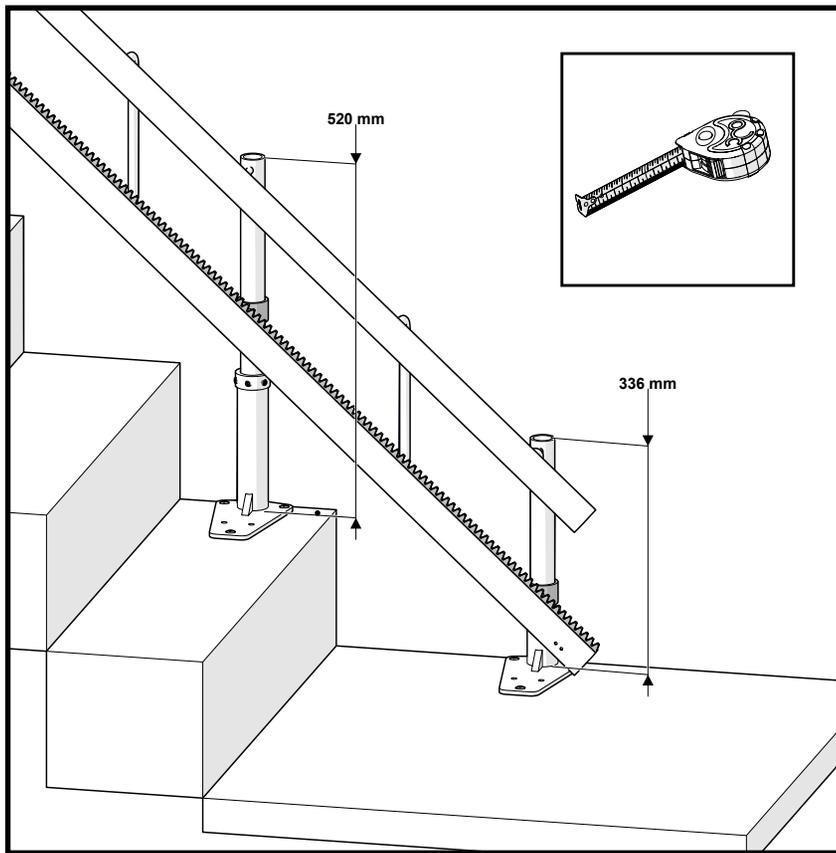
Now the rail is assembled check the heights of the stanchions and bases. These measurements are a guide, due to uneven stairs the numbers may not be exact.
