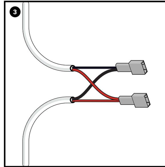
Connect the cables together as shown and crimp into the female spade terminals.
