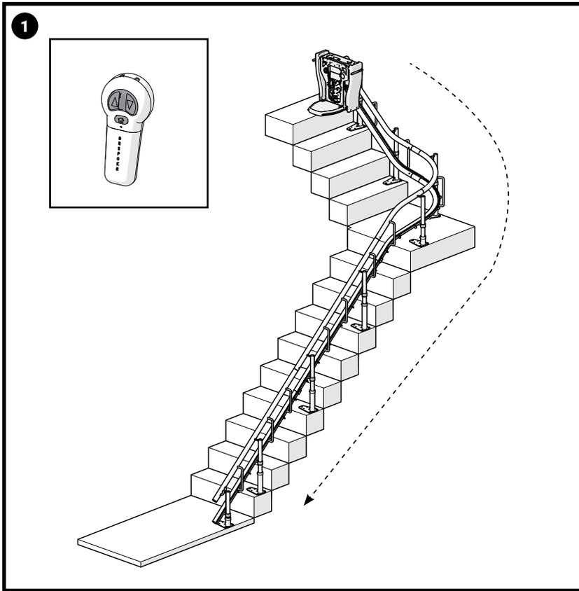
To locate the bottom charge point position use the remote control to drive the carriage to the lower part of the rail.
