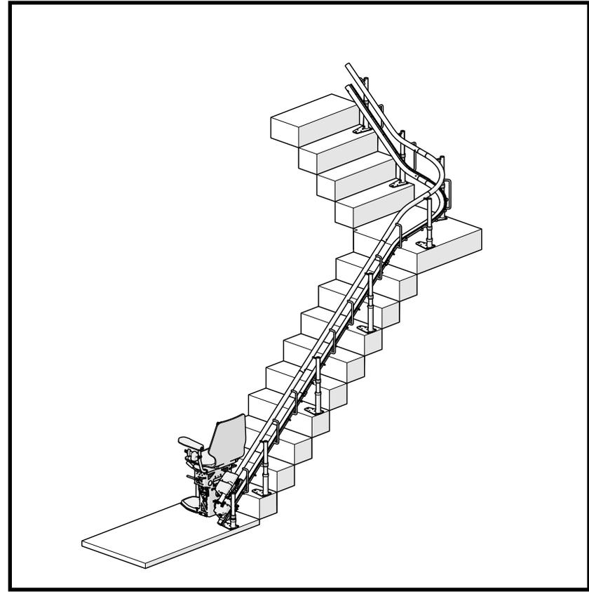
The lift should be positioned on the bottom charge point.
