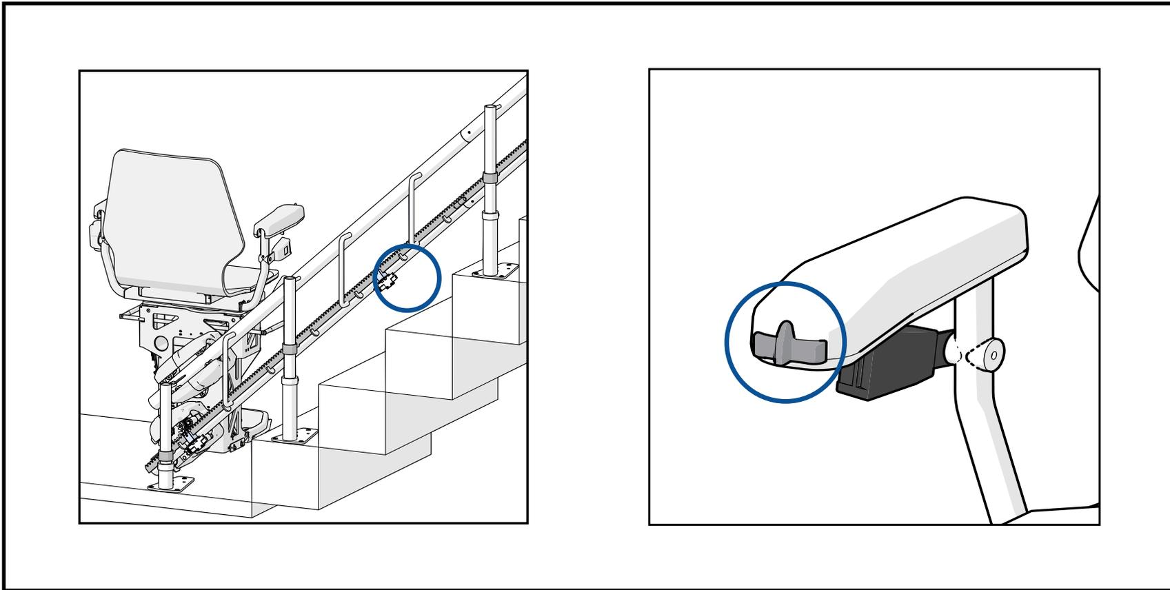
If your stair lift has an intermediate charge point, when running the stairlift upwards the stair lift will stop on this charge point.
