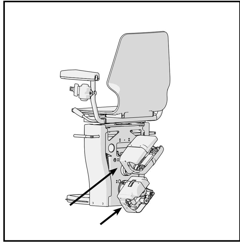
Continue the safety checks on the top and bottom skate safety edges as shown in the diagram.
