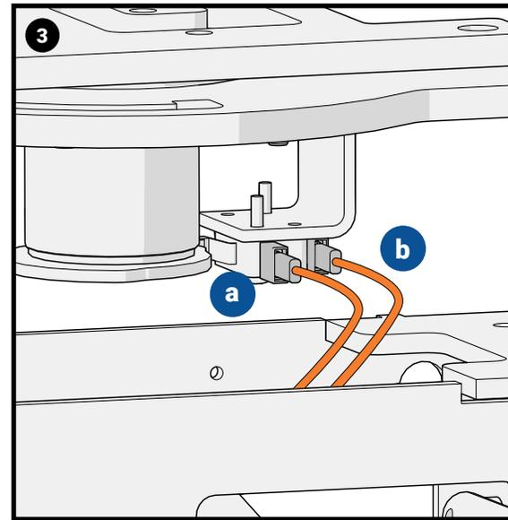
Connect the two cable terminals to terminals **a** and **b** on the Swivel Assembly Switch.
