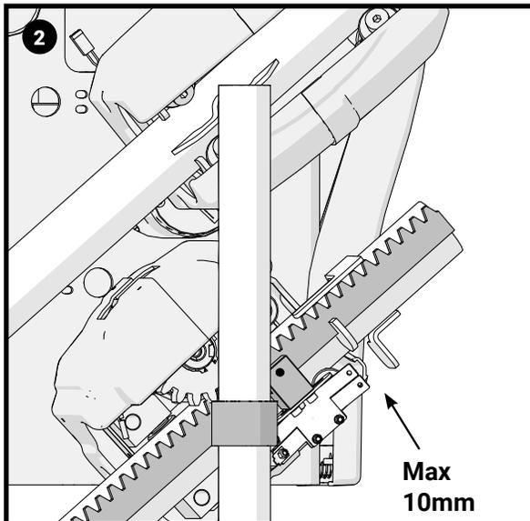
As with the lower end stop, a gap between the end stop and bottom skate covers should be a maximum of 10mm. This is to ensure the carriage will still charge should the carriage slightly overrun.
