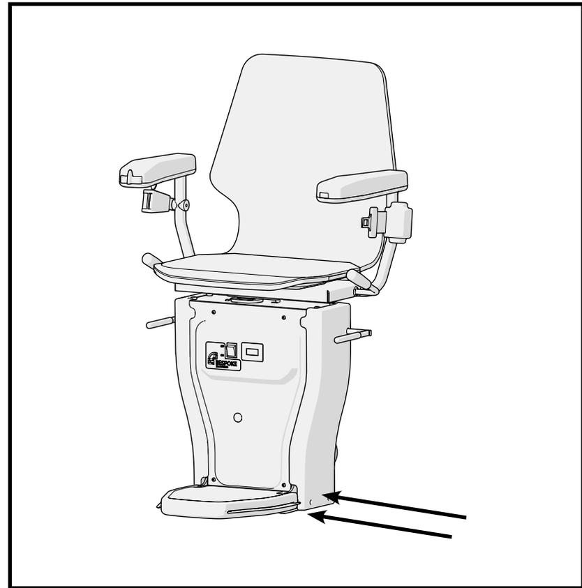
To test the function of the front and side panel safety edges, run the carriage in either direction and press each safety edge shown in the diagrams.
