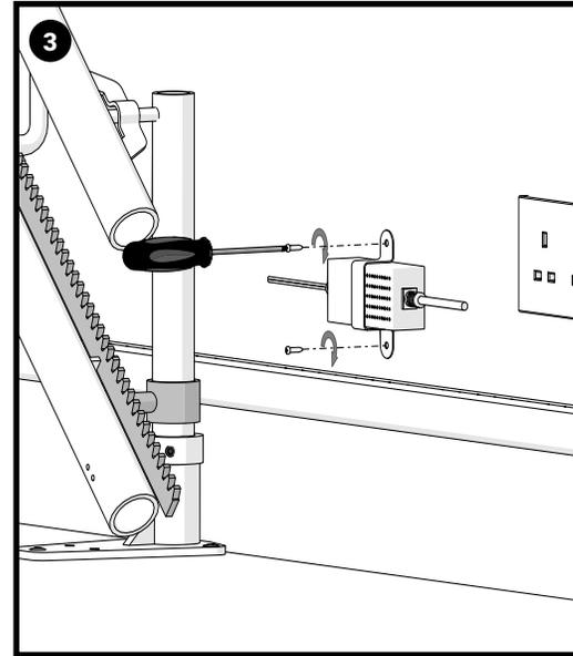
Once the plugs (if required) are inserted. Attach the charger, using the charger bracket, to the wall.
