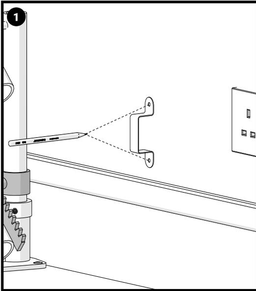
Once a suitable location is found, take the charger bracket and mark 2 holes with a pencil.
