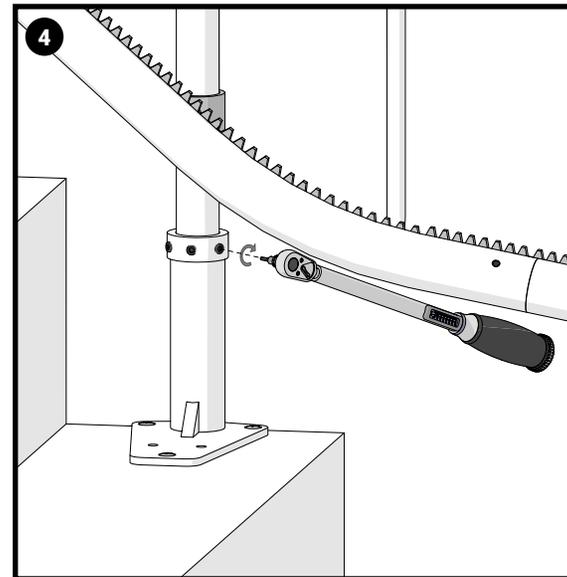
Once the bases are fixed tighten the grub screws to 20Nm. Repeat the process for each base moving up the rail, checking the rail position, until all the bases are complete.
