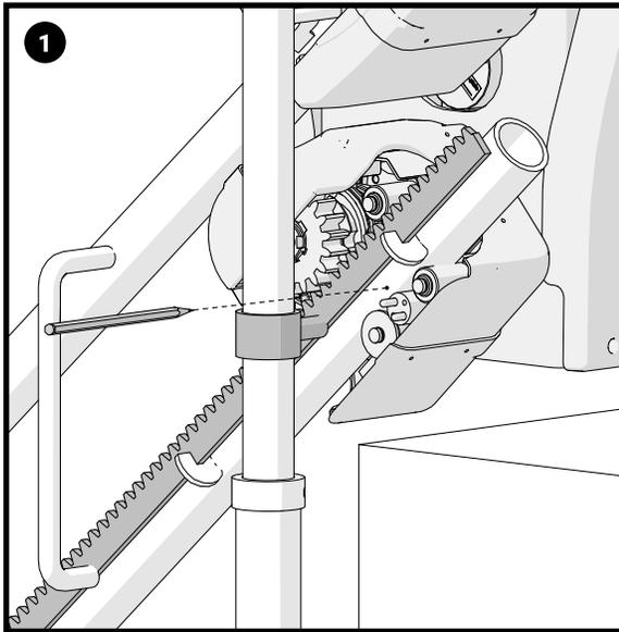
With the carriage in the desired position mark the position of the charge pins located on the bottom skate. Mark this position with a pencil.
