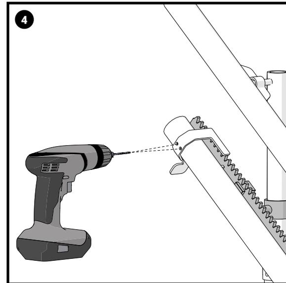
Using a 4mm drill, create a pilot hole for the fixing screws.
