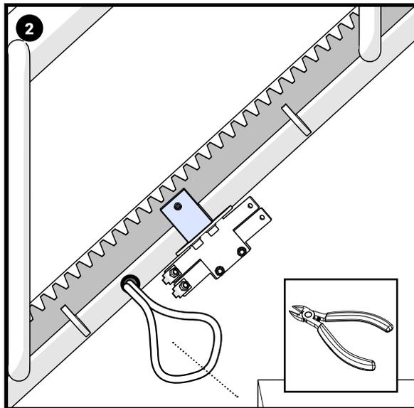
Feed the cable through the hole, ensuring enough cable is available to connect to the charge point.
