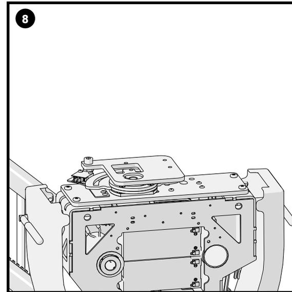
The Powered Swivel Unit is now assembled.
