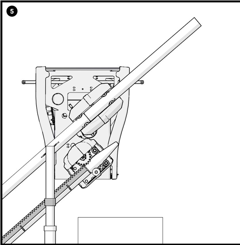
Gently lower the carriage to rest the pinion onto the rack. Keep the loading bar and cone in place.
