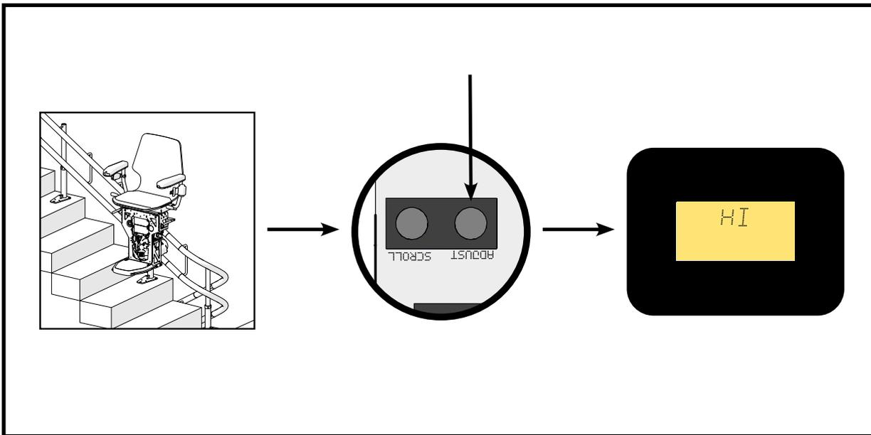
Once the carriage is fully out of the bend, stop the stair lift, press the '**ADJUST**' button and the LCD will display '**HI**'.
