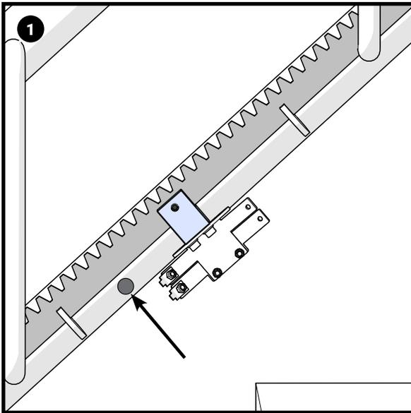
If the rail has an intermediate charge point to park the stair lift in a position other than the top or bottom, locate the pre-drilled hole at the location specified on the installation drawing. Attach the charge point using the provided grub screw.
