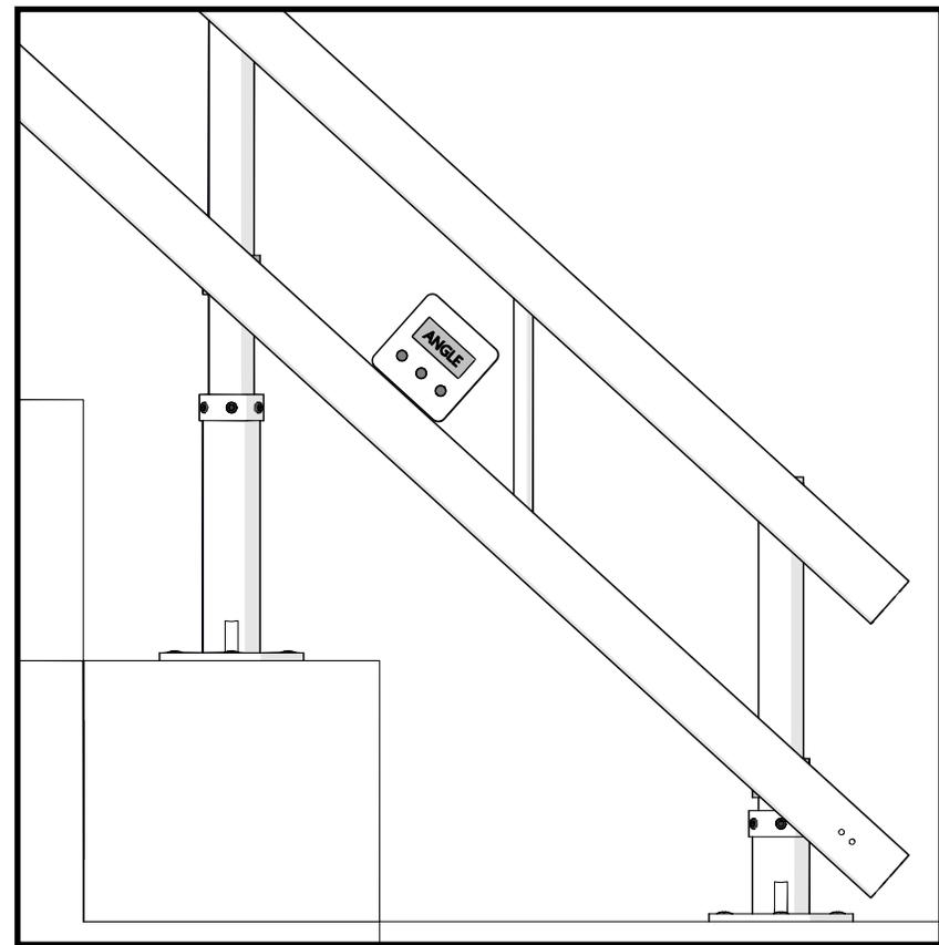
Check the angle of the stairlift rail using a digital angle finder. The angle of the rail should be used as a guide and closely correspond with the installation drawing.
