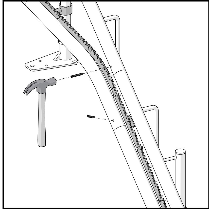
Pins should be flush with stair side of rail. Take care not to damage cable when inserting pins by looking through the hole to see if the cable is not in the way.
