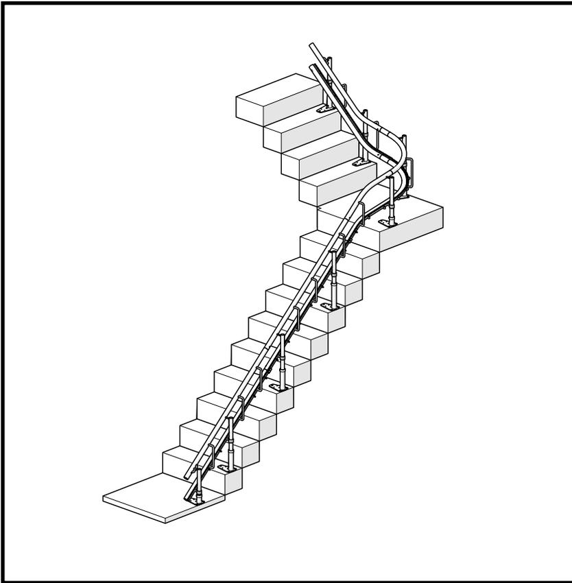
The rail should now be in an approximate position, before the rail is fixed to the stairs the clearances and angles must be checked to ensure the carriage runs correctly.
