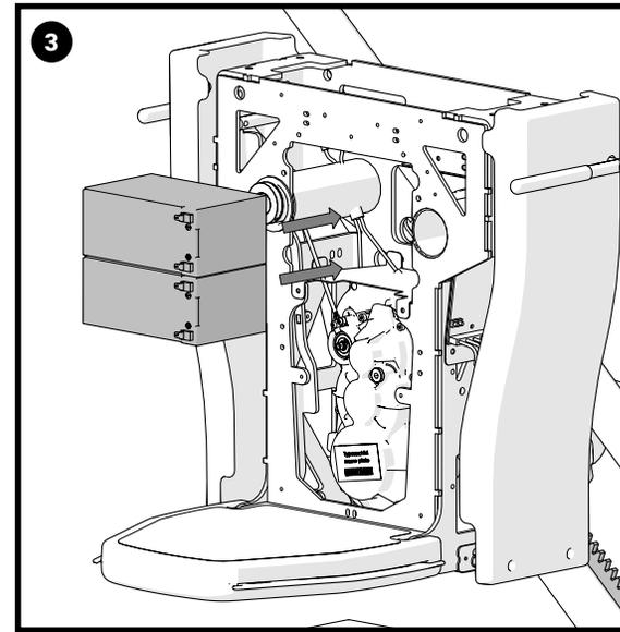
Carefully insert the batteries as shown into the battery tray, being careful not to damage any cables.
