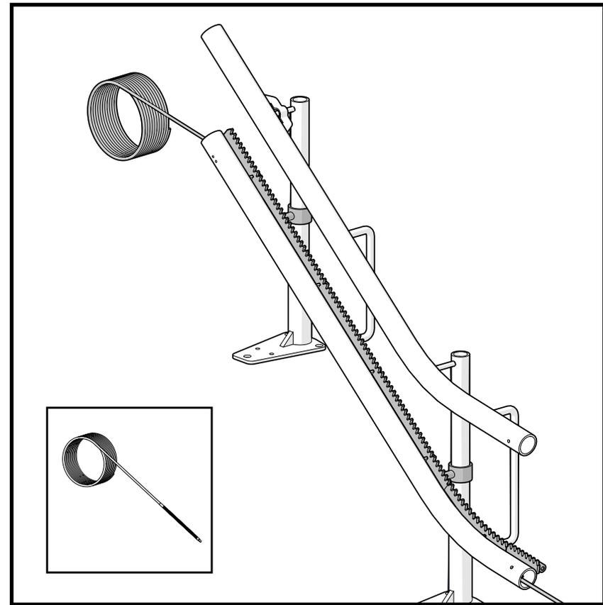
Feed your cable puller into the bottom tube of the top section of rail and feed down through all the sections of the rail until the bottom is reached.
