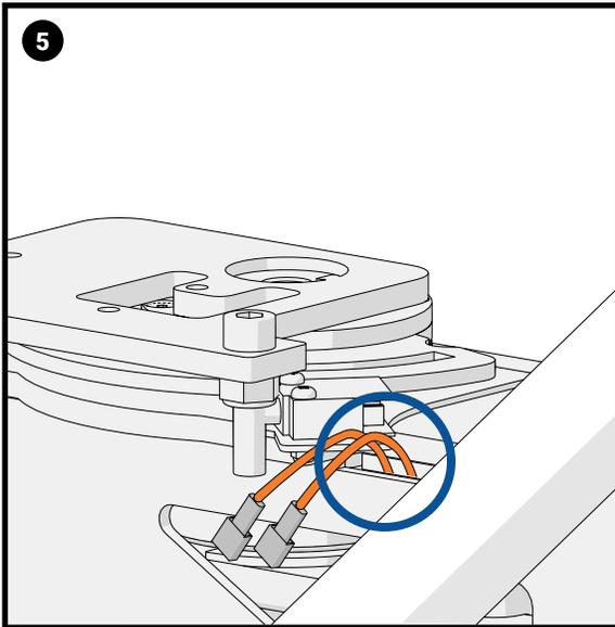
Lower the powered swivel unit onto the chassis frame.
