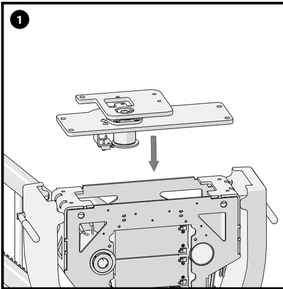
Position the Swivel Assembly onto the Carriage.
