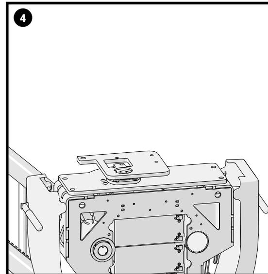
Carefully place the swivel onto the carriage body ensuring the cables are not damaged.
