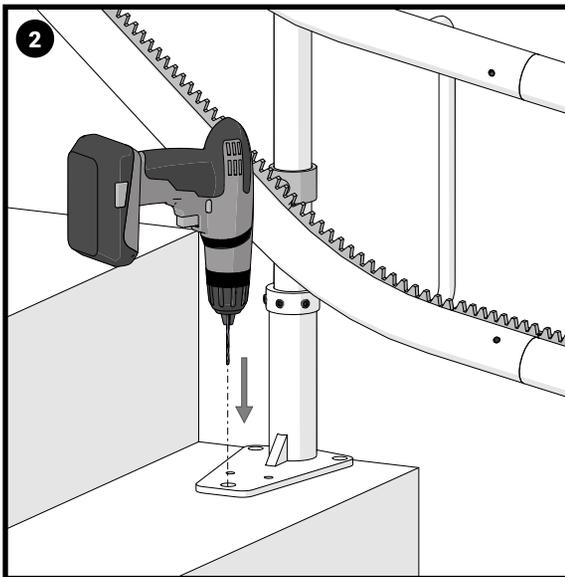
Start fixing at the bottom base. If the stairs are made of a material other than wood drill each of the 3 base holes using a 5.5mm drill bit and insert red rawl plugs. Wood stairs require no drilling.
