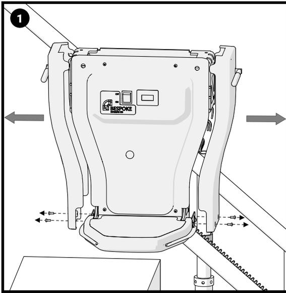
Carefully remove the screws from the side panels and remove. Store carefully to one side.
