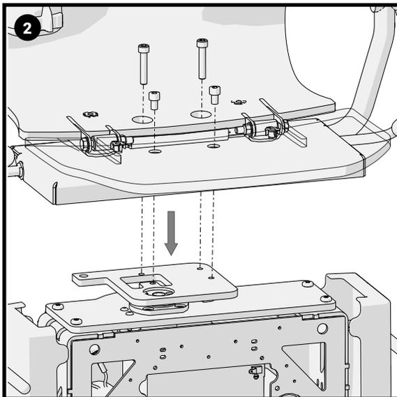
It is important that, with both the powered and manual swivel types, the swivel boss is in the front facing position when locating the seat to avoid misalignment and de-synchronization.
