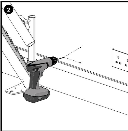
Using a 5.5mm drill bit, drill 2x holes for the wall plugs should they be required.
